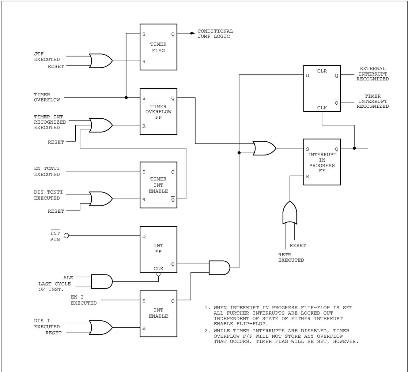
Figure 11. Interrupt Logic
