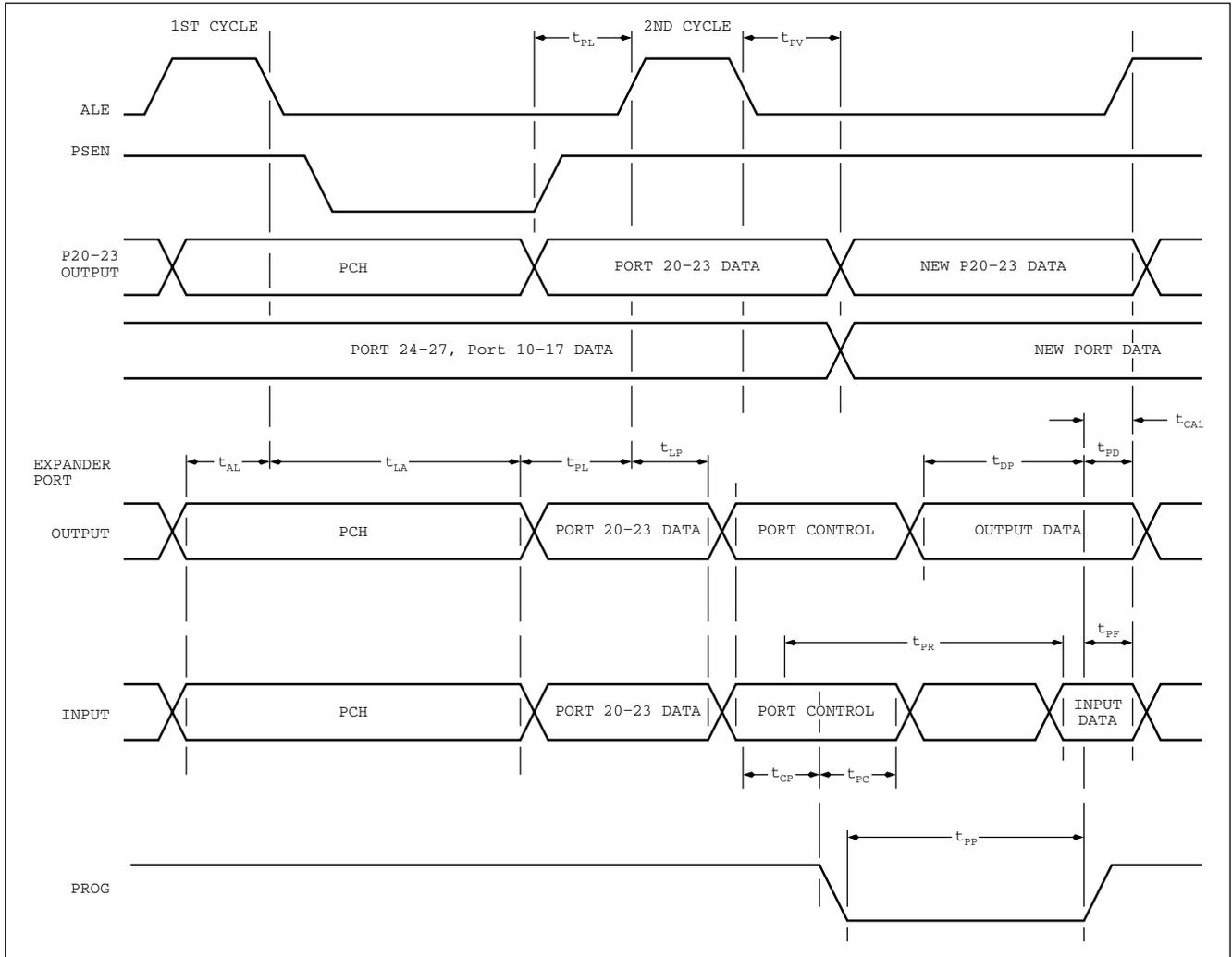
Figure 22. Port 1 / Port 2 Timing Waveforms
