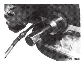
10 Pull off crankshaft sprocket with an extractor.
